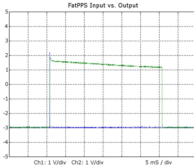
The output pulse is about 30 milliseconds long.
