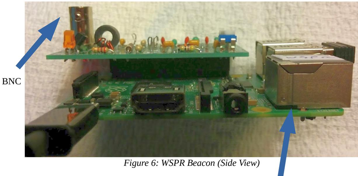
*Figure 6: WSPR Beacon (Side View)*
