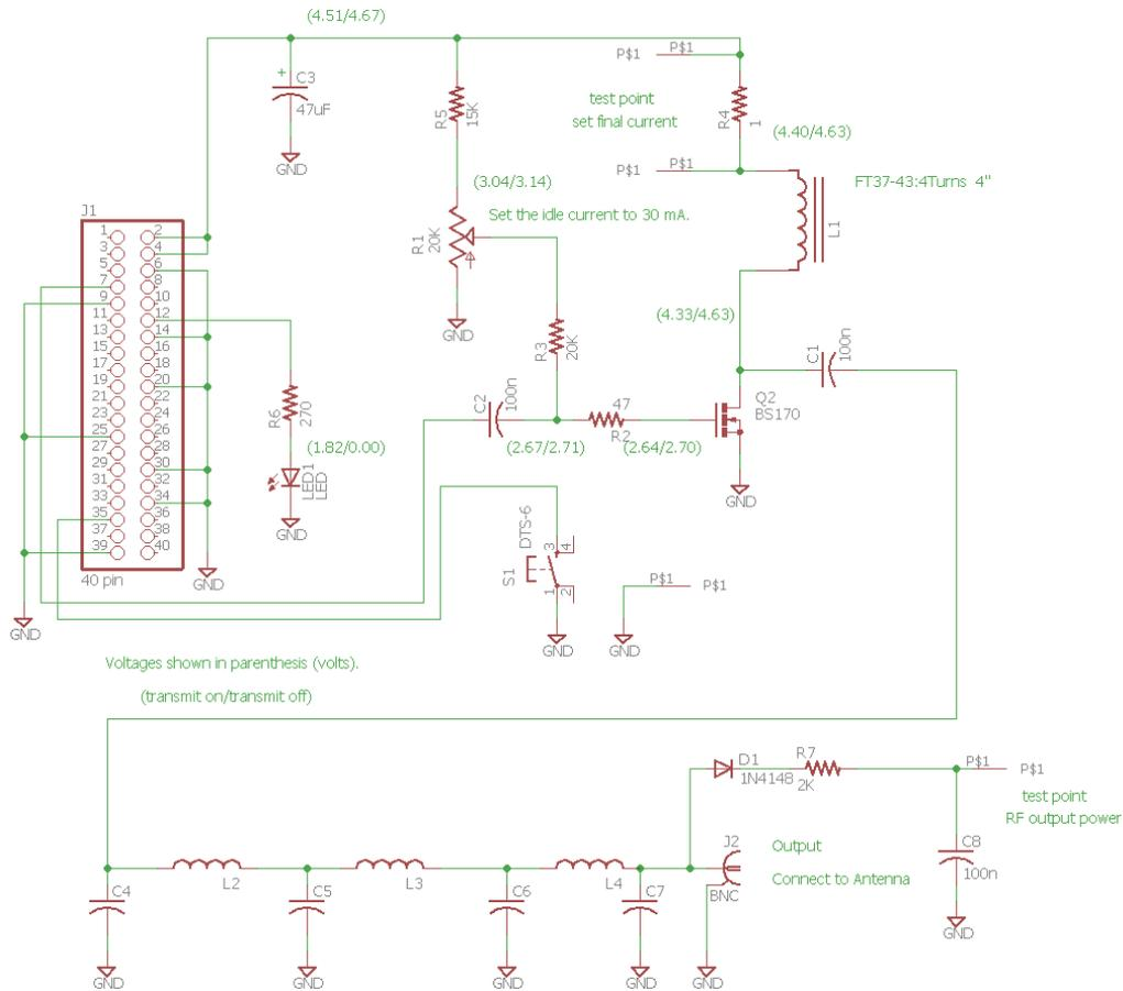
Figure 10: VW Schematic
