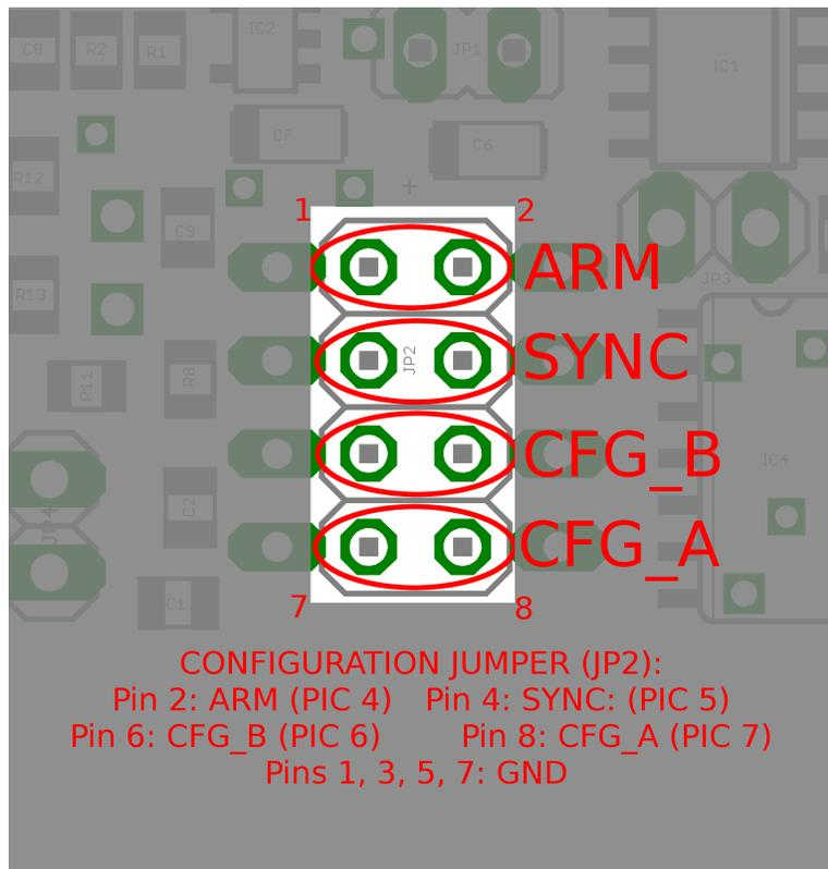
The firmware shipped with the T2-Mini (chip labeled “TVB PD17”) uses the CFG\_A and CFG\_B pins to program the input frequency (for 1 PPS output) as follows:
