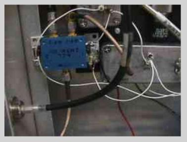
Input PIN diode switch and the RF output N jack.
