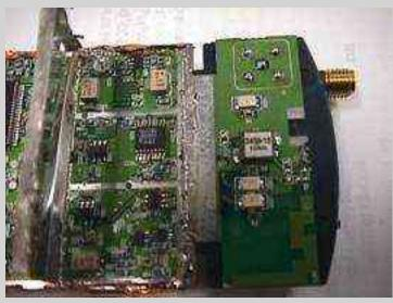
Alternate view. The 6-pin IC sorta in the middle is a <u>NEC UPG152 GaAs MMIC</u> <u>switch</u>. You can tap it's control lines to control an external amplifier.
