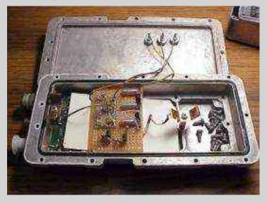
Picture of the transmit/receive control logic boards and the voltage regulators. Once again, housed in an old California Amplifier MMDS downconverter case. +15 VDC comes in through the top via a 1000 pF feed-through capacitor. The transmit/receive control logic from the WaveLAN card enters via one of the F connectors on the right side. The +5 VDC on transmit and +9 VDC on receive signals leave the case through standard feed-throughs (non-capacitor).
