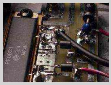
Alternate view to show how the Vapc and Vdd lines are supported in the air by the 56 pF ATC capacitors and the little jumper wires to connect them back to the rest of the circuit.
