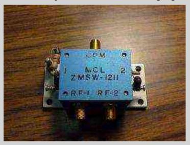
WaveLAN side PIN diode switch module. This is a Mini-Circuits ZMWS-1211, and was purchased from <u>Fair Radio</u> for \$20. The RF connectors are SMA, and the switch logic is +5 VDC @ 2 mA. They are good up to 2.5 GHz.
