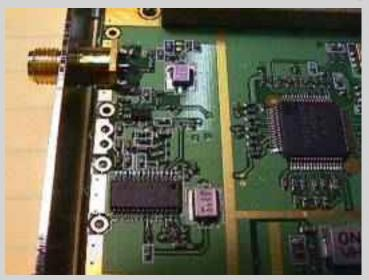
RF power amplifier, standard PRISM2 based hardware.
