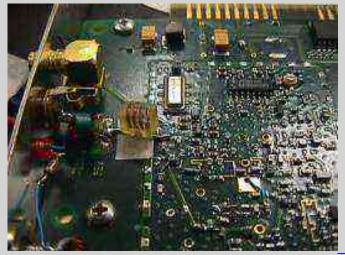
Amplifier's DC Power insertion point inside the
