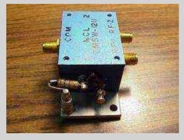
Control line #1 (RF port #1 control) shown. Along with the 100 pF mica bypass capacitor,
