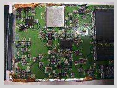
Shown are the HFA3524 dual frequency synthesizer and the associated oscillators and VCOs. Off the to right is the AM79C930 PCnet mobile wireless LAN MAC controller, the 128k flash RAM and the 32k SRAM.
