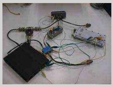
All the modules sorta put together. Please don't use alligator clips, I'm a professional. The male SMA jumper cables are from <u>Down East Microwave</u>.
