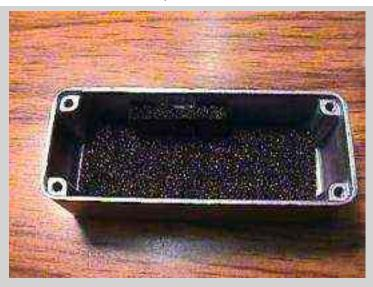
I lined the insides of *all* the cases with that anti-static foam you can buy at Radio Shack, part number 276-2400. Theoretically, this will absorb stray RF inside the case and help improve the circuit's input/output isolation. Or maybe I just smoke \$2 crack....
