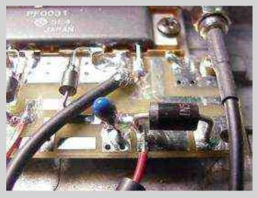
Closeup of the RF output side and the Vdd line. You can see the decoupling capacitors and the idiot diode.
