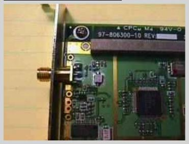
Antenna connector. Reverse polarity SMA connector. Diversity antenna switching is done by applying the DC control voltage via the coax to the included external diversity antenna.
