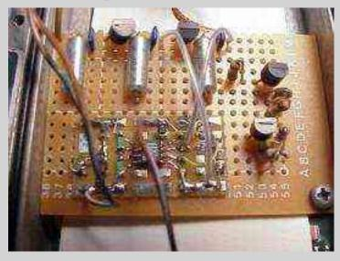
The 78L05 in shown in the top left, 78L09 is top right. The HRF49093 MOSFET is mounted on a surface mount carrier called a Surfboard. I used surface mount parts in the transitor switching logic for simplicity. *Ignore those two transistors on the right hand side*.
