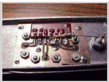
Closeup of the PIN diode module. You can see the bias resistor and ferrite bead floating in the air. The bias line passes through a regular feed-through (non-capacitor). RF connectors are SMA, with the teflon covered pin (ala the 33LNACK), the connectors are also available from <u>Down East Microwave</u>.
