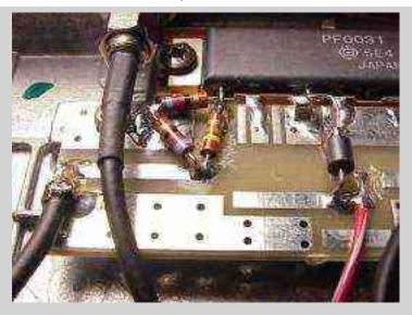
Closeup of the RF input side and the 20 dB attenuator. Should probably use surface mount resistors in the attenuator pad, but they won't handle the fairly high RF input power. You can also see how the circuit board was cut to isolate the Vapc line.
