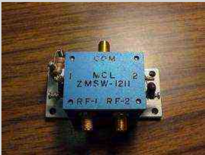
WaveLAN side PIN diode switch module. This is a Mini-Circuits ZMWS-1211, and was purchased from Fair Radio for $20. The RF connectors are SMA, and the switch logic is +5 VDC @ 2 mA. They are good up to 2.5 GHz.
