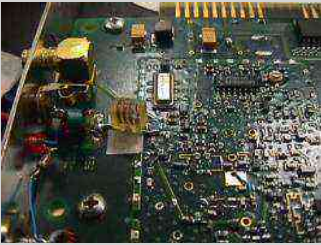
Amplifier's DC Power insertion point inside the
