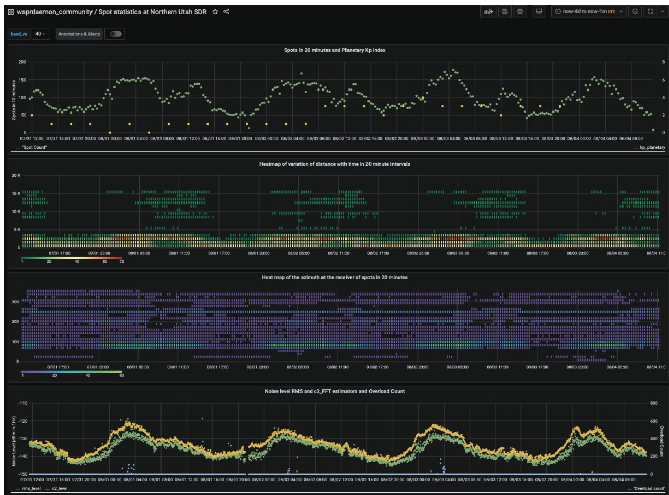
Figure 5. An example Grafana Dashboard that combines simple time series graphics from three sources with heatmap representation of data. The data spans four days for 40m from KA7OEI-1, a KivisDR at the Northern Utah SDR site. The top panel shows the number of spots received in 20-minute intervals in green, with three-hourly estimates of the planetary geomagnetic disturbance index Kp in yellow. The second panel is a heatmap of the number of spots in 20-minute intervals within 1000km distance bins out to 20,000km. The third panel shows azimuth at the receiver in 15° and 20 minute bins. The bottom panel shows the c2_FFT and RMS noise estimates with a distinct diurnal pattern.
