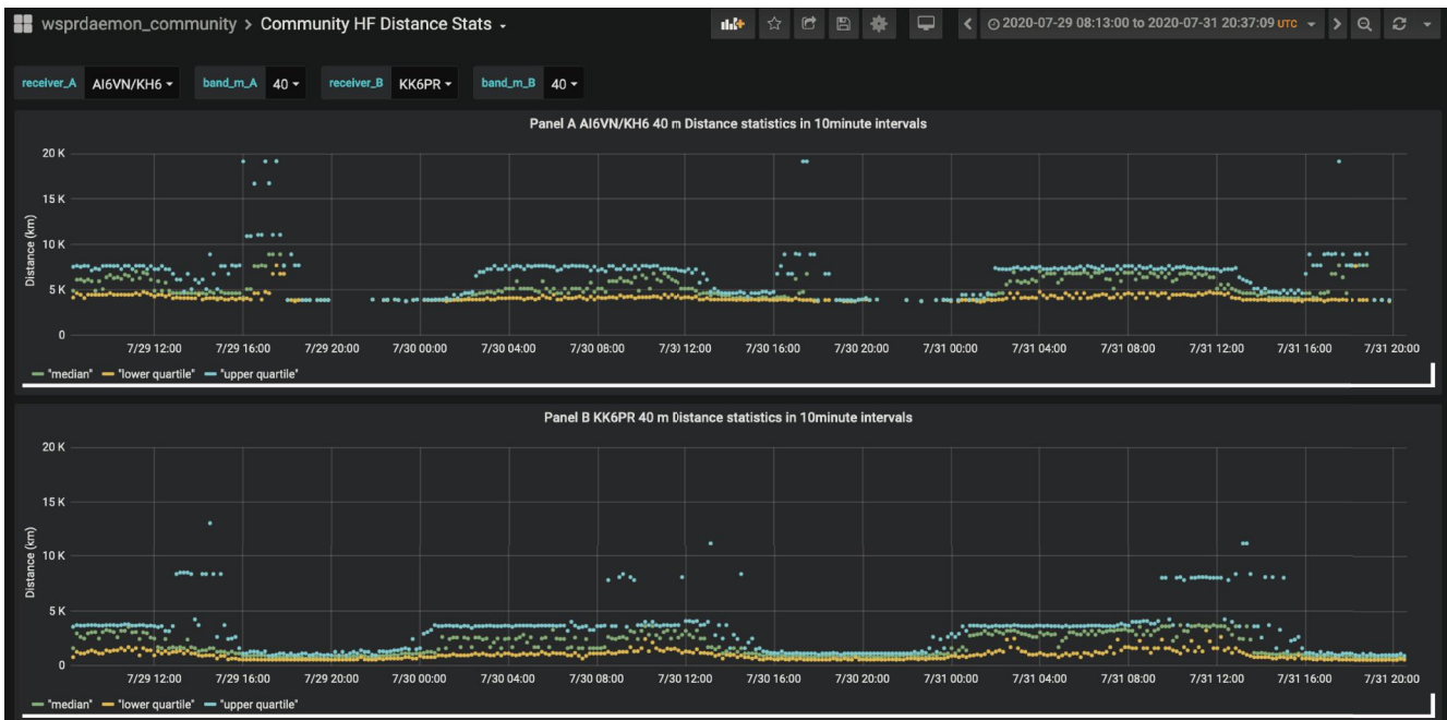
Figure 4. Grafana Dashboard that enables a user to compare distance statistics in 10 minute intervals (lower quartile, median, upper quartile) for two receivers and two bands. As in this example, a comparison may be between two different receivers on the same band, but can also be used for the same receiver on two different bands. Pull down options at top right set the time span and the user can save or export the plot, or save the data in csv or json formats.
