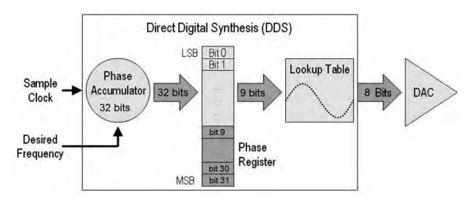
I just adapt it for an Arduino to generate WSPR, CW, PSK and QPSK 31,63,125 modulations. I use 32 bits phase accumulator and 9 bits pointer to lookup table. The PWM is used as DAC (Digital Analog Converter)
