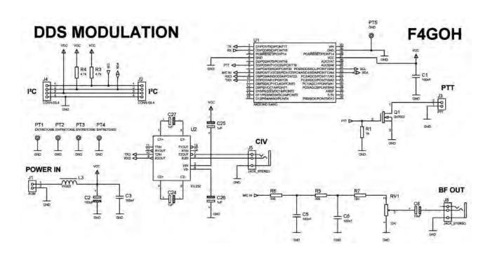
The DS3231 is used to synchronize time transmission(J4). Arduino Nano generate Audio frequency around 1500Hz (J3). RV1 adjust Audio level Output. CIV system is a software serial via Max232. That's control VFO and PTT (J5). There is also another PTT output (2N2007 in open Drain J3). Power supply is 5 Volts, there is no DC/DC converter.
