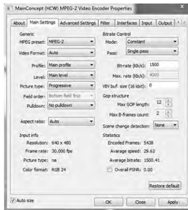
Properties of MainConcept video encoder filter using ConstantBitRate (CBR)
