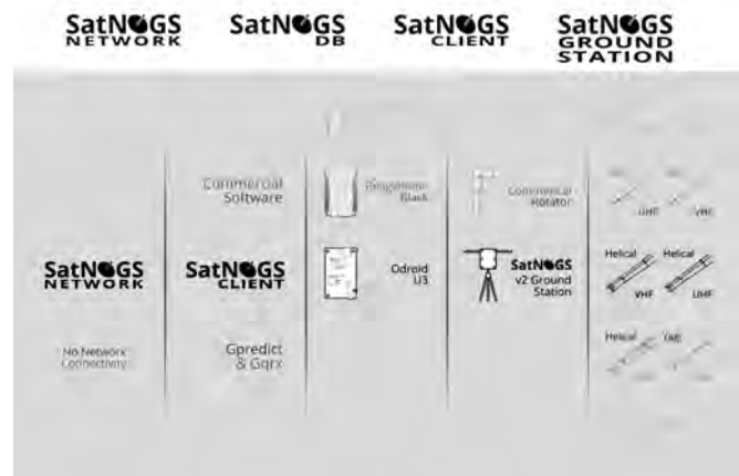
Fig. 3. The four sub-projects are designed with a modular approach with well-defined interfaces, allowing the ability to relatively easily interface with existing ground stations.
