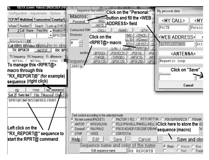
It will remain to push on the <TX> button to send the RPRT@ command to the other Ham.
