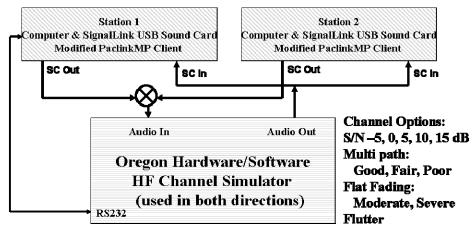
Figure 3. Protocol Testing Setup using HF Channel Simulator.
