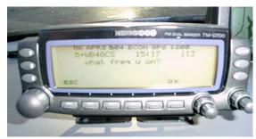
Figure 8. The front panel APRS message capability of the Kenwood D700 radio. Messages can be up to 64 characters in length.
