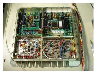
Photo 9. The KPC-3+ TNC system with Hamtronics TX and RX inside the ANDE comms tray.
