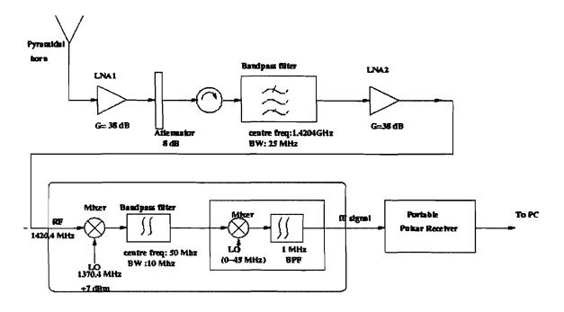
Figure 2:Block schematic of the receiver system for the reference signal. Portable Pulsar receiver is used for acquiring data and formats data to transfer into PC.
