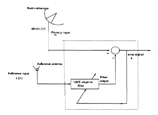
Figure 1:Schematic of RFI mitigation using adaptive interference cancellation
