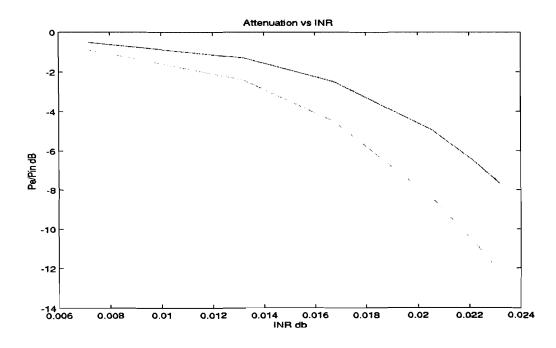
Figure 3:Simulation results of adaptive interference cancellation, Attenuation vs INR. The results show that constraining the bandwidth of the reference signal, the suppression of RFI improves with SNR
