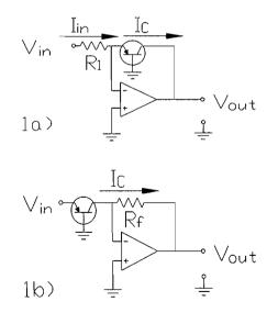
(a)  $V_o = -(0.025) \ln(V_{in}/I_{eb}R_1)$ (b)  $V_o = -R_f I_{eb} \operatorname{antilog}(V_{in}/25mV)$
