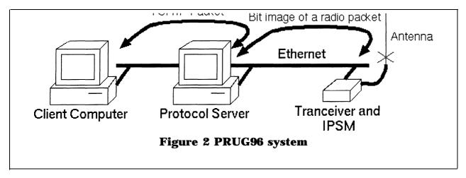
Creates bit images of the packet to be emitted. Then, the PS encapsulates the bit images in a UDP packet and sends to the IPSM. After the IPSM receives a UDP packet, the IPSM removes IP/UDP header from the UDP packet and hands them to the transceiver. Finally, the transceiver emits the packets on the air.
