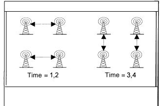
In this situation, pairs of stations would share hopping sequences. For timeslots 1 and 2, the upper pair of stations would share a hopping sequence. The lower stations would also share a different hopping sequence. In Timeslots 3 and 4, the stations on the left would share a hopping sequence, and the stations on the right would share a different hopping sequence.
