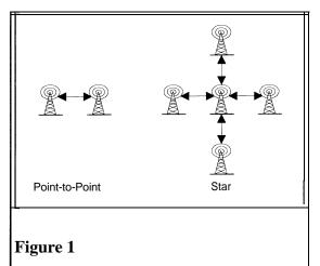
However in a spread spectrum situation this is not a good use of resources. This if especially so in the case of the star configuration. The utilisation can be defined as the time spent by all stations transmitting or receiving divided by the total time. In the start configuration with four stations, the utilisation becomes 16/40 or only 40%. This means that on average 60% of each stations time is being wasted.'
