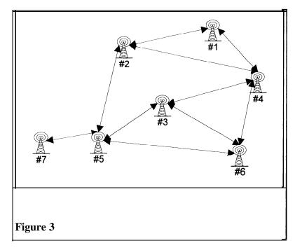
It can be seen that most of the time pairs of stations can communicate without any problems. However when stations 5 and 7 are communicating not all of the remaining 5 stations may communicate. This problem can only be minimised, but never eliminated.
