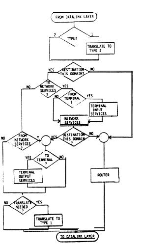
Figure 4. GENERAL DATA FLOW IN STATION NODE
